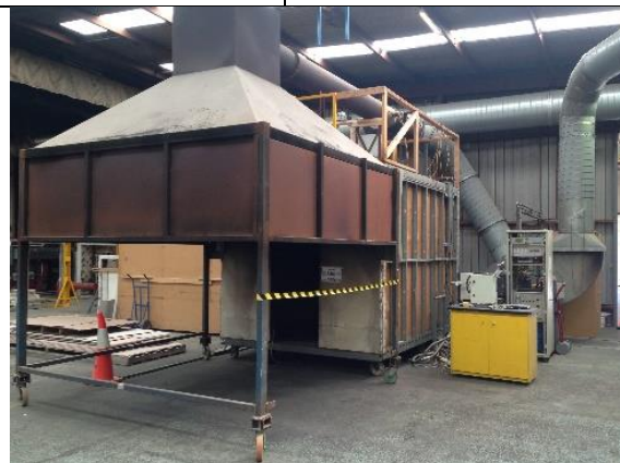
Photo of the ISO 9705 test rig.
