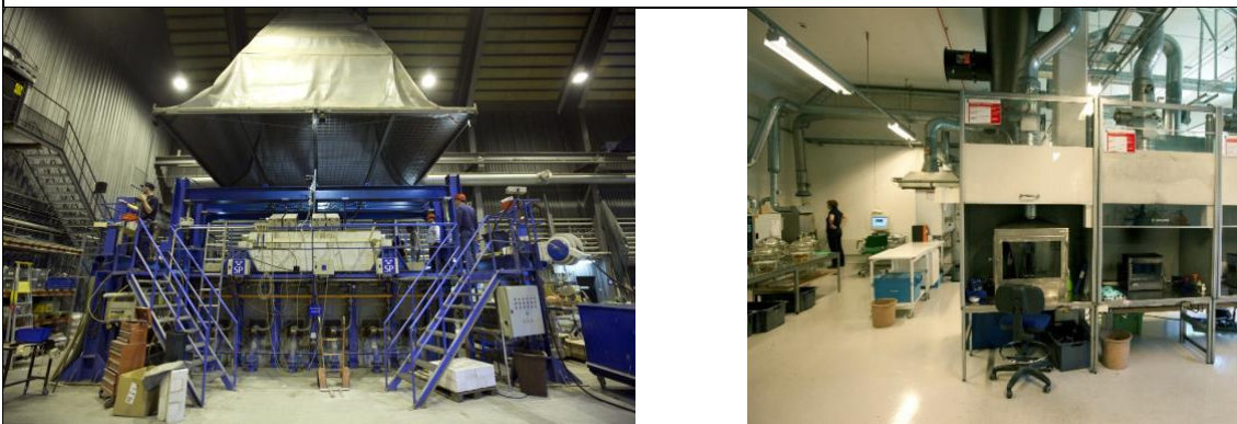
Figure 17: Horizontal furnace for fire-resistance testing (left) and small-scale testing facilities (right).
