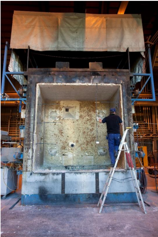
Figure 15: Vertical furnace for fire-resistance testing.
