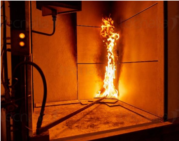
Figure 14: SBI (single burning item) testing of an external cladding system.
