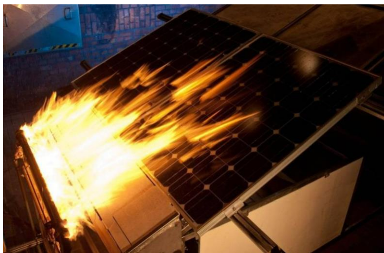
Figure 6: Spread of flame test.
