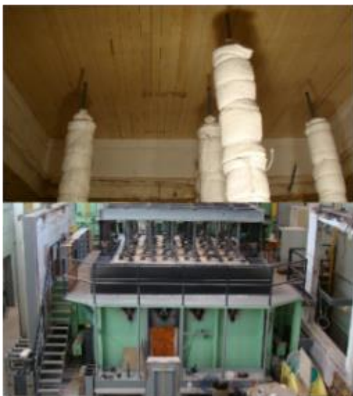
Figure 5: Photographs of fire-resistance testing facilities. Thermocouple trees installed in a test room built with massive timbers (top) and floor test furnace (bottom).
